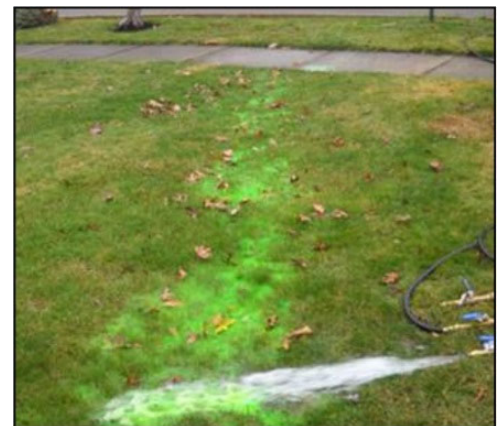
Ponding over sanitary lateral during rainfall simulation
