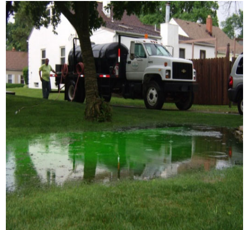
Ponding over sanitary sewer and sanitary lateral during rainfall simulation
